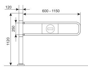
An electronic gate Porta'e Infra is steering by photoelectric cell without lighting. Gate can be available in two option: right or left - opens in right side or left side. The gate opens automatically in the direction of entry as you approach it. The gate closes also automatically.
